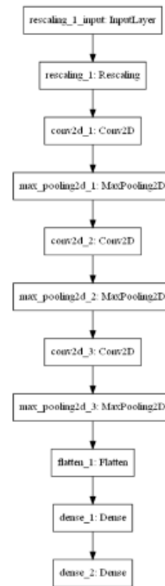
Figure 5-7. First Model Architecture for ModelNet10
