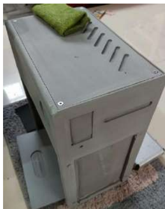
Gambar 5. 13 Proses Finishing Body Chamber dan pengecatan
